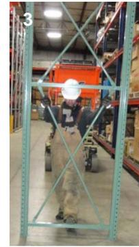
Photographs 1, 2 and 3 show a Truss being raised to its upright position. Make certain the Truss Base does not slide by placing a foot on the Bottom Horizontal brace.
